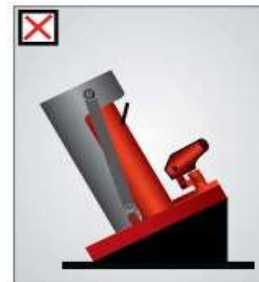
Keep the Jack even at all times on level ground while loading.
